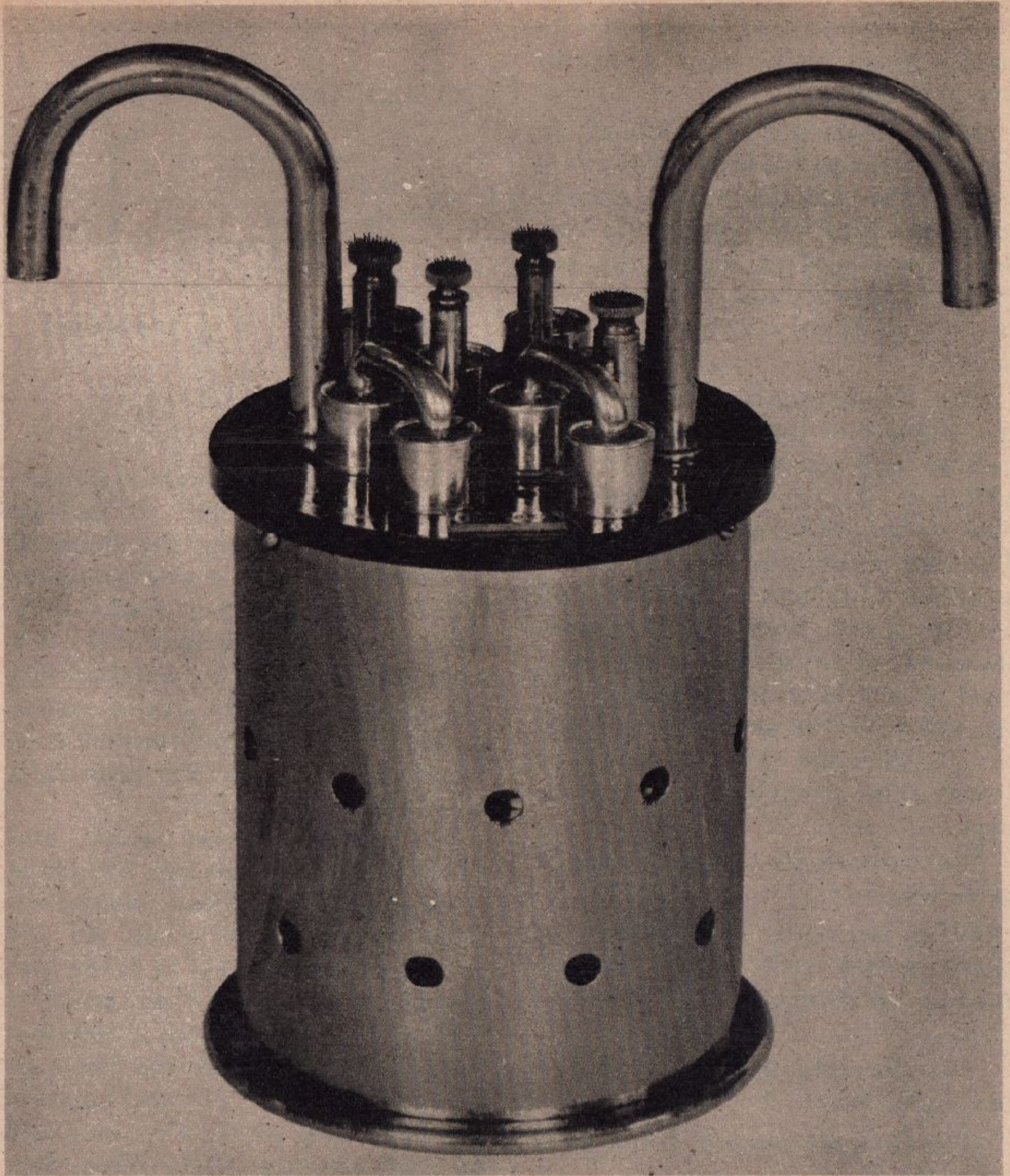
G.E.'s. 10:1 ratio standard, used in conjunction with the precision bridge for checking primary standards. Mercury cups and mercury amalgamated arms on top provide an easy means of changing the ratio, and at the same time insure good contact.
