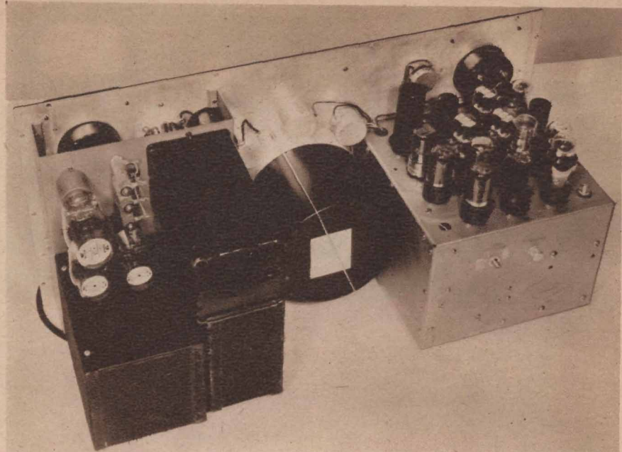
Interior of the ultra-high frequency generator, with shield cans in place. On the left is the power transformer, rectifiers and filters; the oscillator circuit elements are in the large can at the center. At the right are voltage regulator tubes, and the pulse-generation circuits and modulator tubes.
