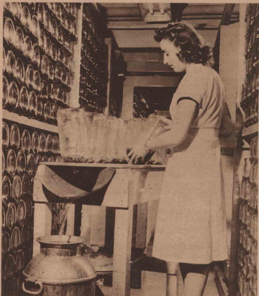
The penicillin produced by the mold's life-processes appears in the liquor, here being harvested from "ripe" cultures. It's a slow, expensive system.
