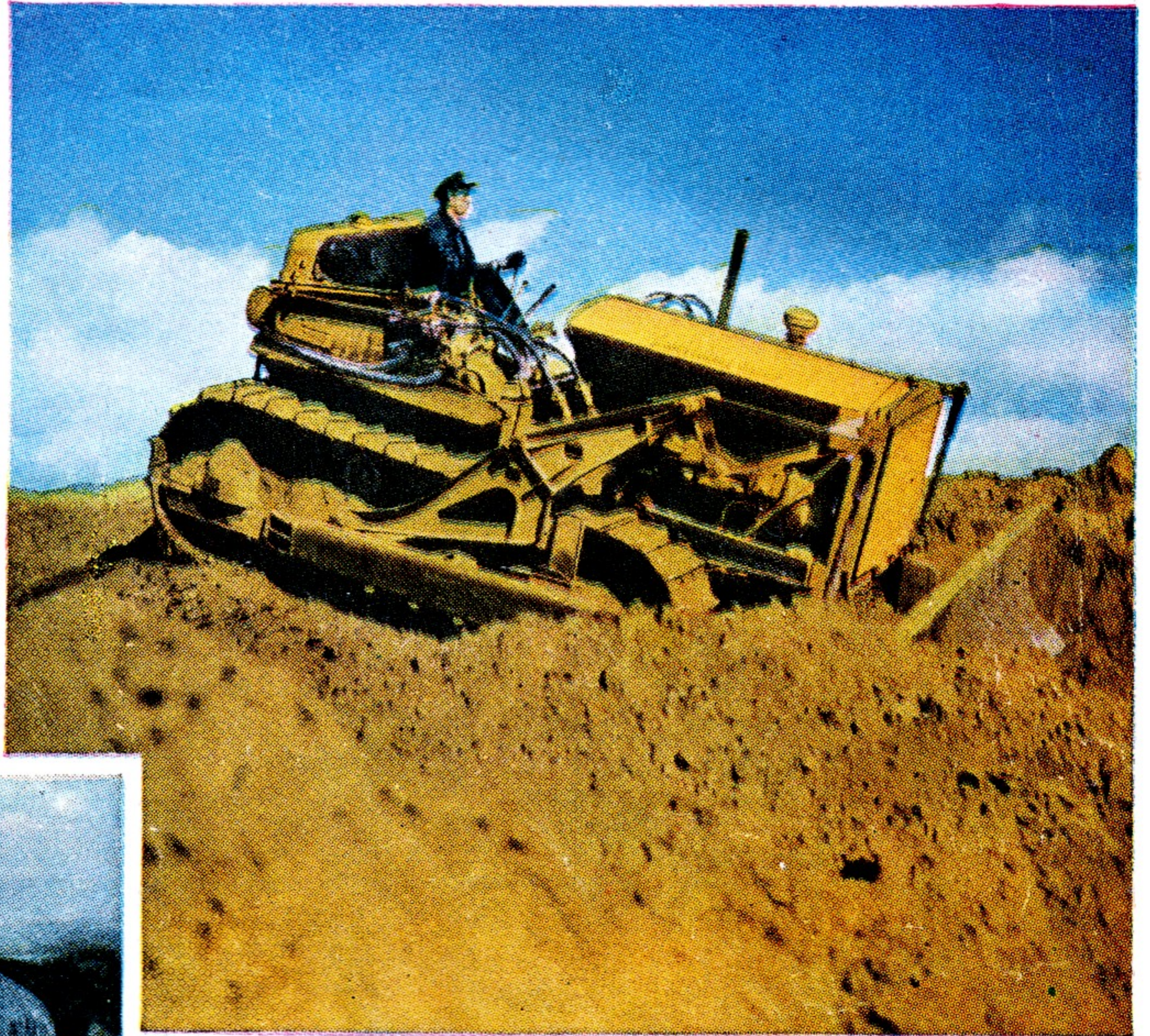
BUILDING A FIRE-BREAK. Operators of these powerful Diesel caterpillars are called “skippers.” McNichols must negotiate treacherous slopes ... as he handles this mighty machine that takes rocks ... brush ... trees in its stride at a steady \frac{1}{4} m.p.h.
