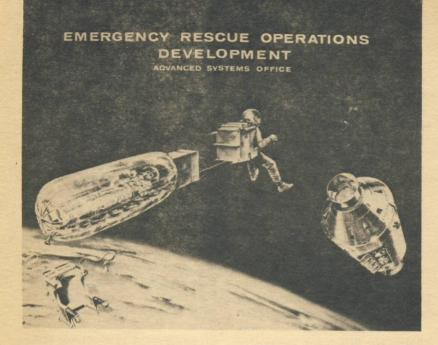
one astronaut. He dons his spacesuit and leaves the crippled spaceship. The disk-shaped heat shield would be assembled with the astronaut sitting in the middle and a silica-plastic foam material filling in an inflated mold. The foam would harden in minutes and the astronaut would strap a small solid fuel rocket motor on his chest.
