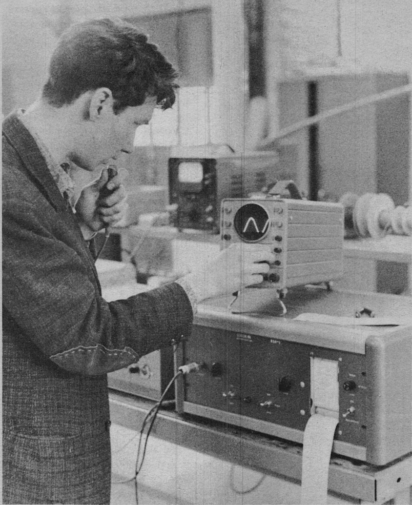
Steve Moshier examining spectrum of the output of the Man-to-Porpoise Translator. The frequency components of the whistle output are broken down and displayed on a sheet of facsimile paper by the Multi-Spectrum-Analyzer.
