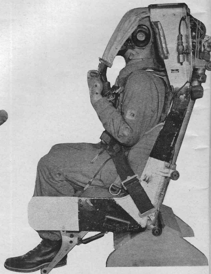
1. The articulated manikin used in automobile crash research, escape-systems testing, and other hazardous experiments is a forerunner of a future dummy space-explorer. All the major human motions are simulated, and the vinyl skin bonded to foam flesh approximates the compression, buckling, and displacement of human flesh. The instrument package carried in the torso is accessible through a chest opening.
