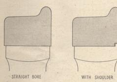
preventing flanging, or the wearing away of the vertical surfaces of flanges. These flanges must never be allowed to get below <sup>15</sup>/<sub>16</sub> of an inch in thickness. Below that point they allow for too much lateral and show a tendency to split switches.
