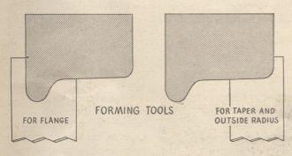
Rigid standards govern flange and tread contour. Too thin a flange results in "nosing," and a tendency to split switches
