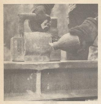
Powder test. Big G crews, supervised by General Roadmaster L. J. Gilmore, have a simple means of attesting the efficiency of their welds. Once the area in question has been dusted with Magna-Flux powder, an electro-magnet (left) is brought in contact with these minute iron filings. Pattern taken by the particles reveals any flaws in the weld or presence of unground seams
