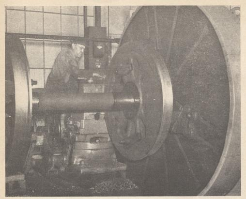
Above: Turning a pair of tires on a lathe takes from 30 to 45 minutes, depending on wheel diameter. Feed range is from 1/10 to 3/10 of an inch per revolution of the face plate
