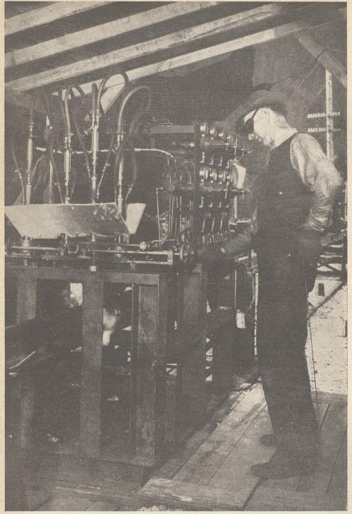
Housed in one of the many wooden sheds that comprise the outdoor assembly line, this multigaged instrument is called the normalizer. By reheating the welded area to between 1500 and 1550 degrees, it relieves the stress and strain produced within the metal by the extremes of pressure and heat that have tortured the steel in previous operations
