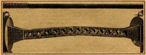
A STEEL COLUMN BUCKLED AFTER A TEST IN THE EMERY MACHINE, A FAULT DETECTOR THAT IS CAPABLE OF EXERTING A PRESSURE OF 2,300,000 POUNDS AND A PULL OF 1,150,000 POUNDS.
