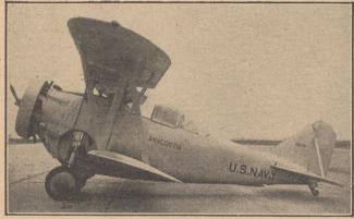
Above: The Navy is buying lots of these new Grummans fitted with the 620 Cyclone engine. This ship does well over 200 m.p.h. and boasts a rare armament, retracting wheels and special equipment for flying deck work with the aircraft carriers.
