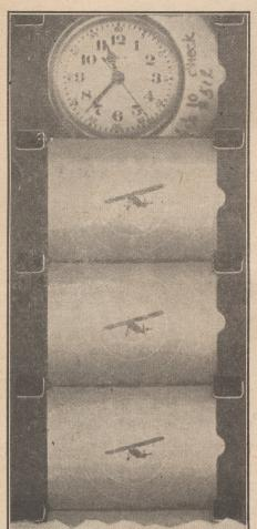
Here's an enlarged section of negative film from a Fairchild camera machine gun. It shows a typical series of photographs. The image of a watch and data card shows at the end of each series of exposures, or bursts of fire.
