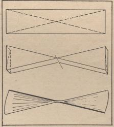
Various steps in the carving of a simple type propeller.
