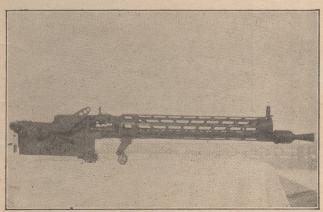
A real close-up of the famous German Spandau machine gun. The strange muzzle-cup on the end of the barrel was a gas-recoil arrangement to speed up the rate of fire. Note the original water jacket, slotted out to allow the barrel to be cooled by air.
