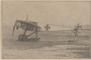
One of the most unusual photographs of a World War ship. This is the little-heard-of Fokker E-2, built late in 1914. Notice that it does not carry fixed machine guns, for the interrupter gear had not then been invented.
