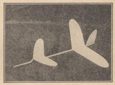
HE easiest way to win an award in a contest is to build a glider. The tedious job of covering a cambered wing with microfilm is done away with, because a glider is solid, not built up, like most indoor models. A glider, however, must be built just as carefully. The most difficult part of making a contest model is designing and adjusting it.
