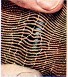
A Note how cords of most tires are bunched and gapped by slender cross-threads. Result: weak spots, "slaeker" cords, overworked cords. BFG cords, instead, are sealed in rubber, with uniform spacing and tension.
