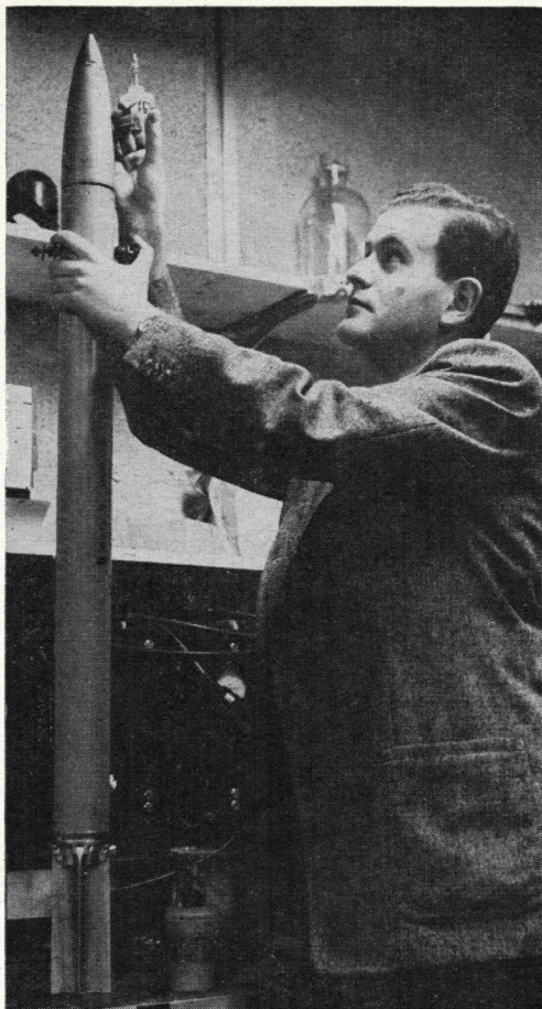
Dr. Fred Singer, MOUSE inventor, with a Rockair rocket and the tiny unit—consisting of a Geiger tube, a sound amplifier, a radio transmitter, and a power supply of 900 volts—which the physicist designed to fit into the 2¾-inch diameter of the Rockair's nose cone.
