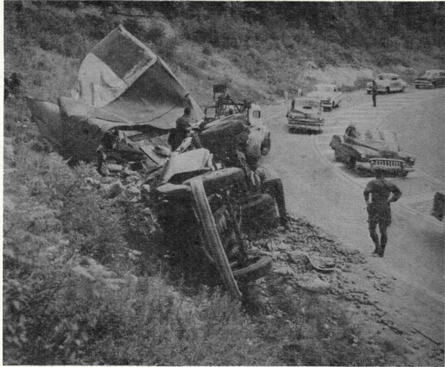
DEATH TRAP on New York's Route 17 features steep hill, then hairpin curve where highway squeezes from four lanes to two for underpass. Truck failed to make curve. Scores of cars have crashed here.
