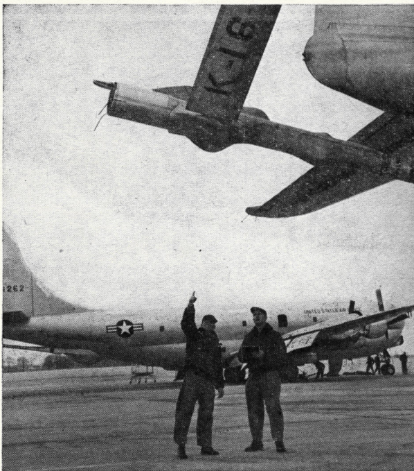
Capt. Doddington and S/Sgt. Barker look over the fueling boom at the tail. It has its own wings and can extend 17 feet.
