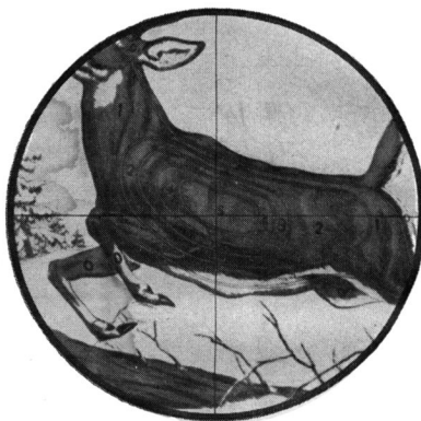
Twenty-five-power target scope sight gives large magnification with a very small field of view.
