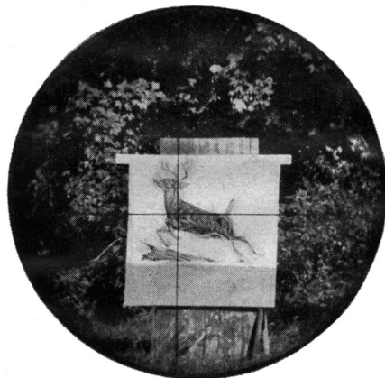
Six-power scope shows larger target, smaller field. Improperly mounted base puts reticle off center.
