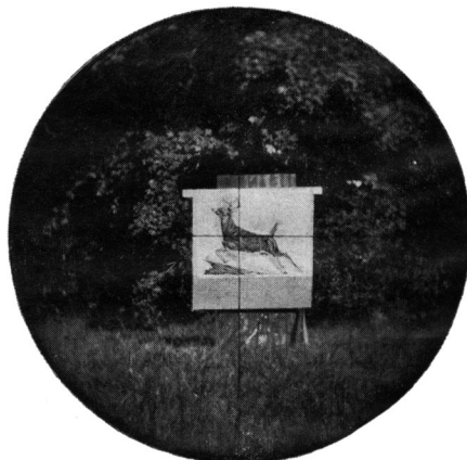
Four-power scope has large field of view so shooter can quickly pick up target that may be in motion.
