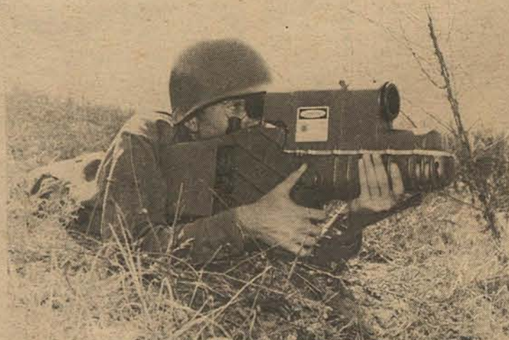
A lightweight laser designator, built by Hughes Aircraft Co., is aimed by an infantryman to pinpoint targets for laser homing missiles and projectiles during an Army test.
