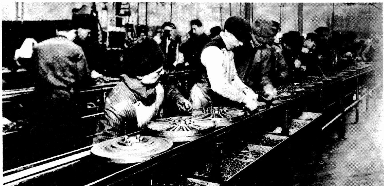
A big step forward for capitalist technology: the first assembly line, Ford's Park Plant, 1913.
