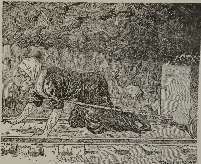
IN ENGLAND'S EARLY NINETEENTH CENTURY COAL MINING WOMEN PULLED THE LOADED CARS OUT IN THIS MANNER
