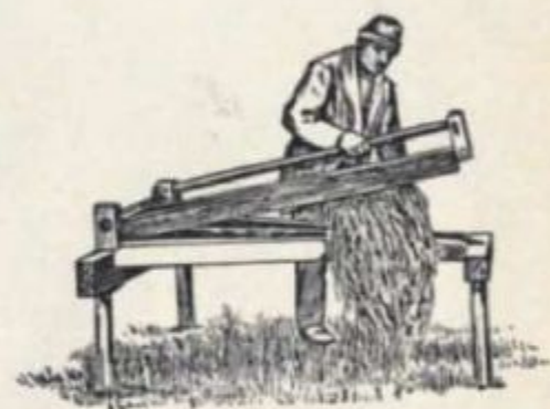
A Kentucky hemp brake, used for reducing the hemp stalks to useable fibre.
