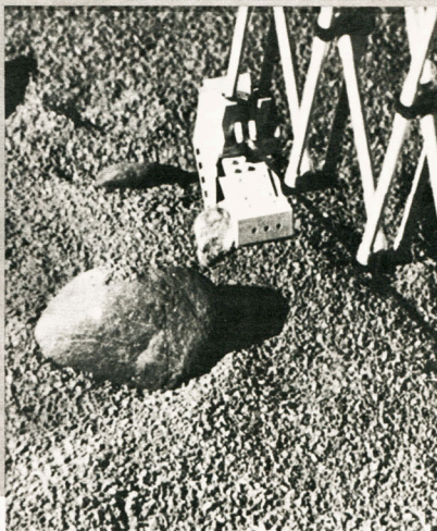
No larger than a man's hand, this steel-tipped dirt scoop was extended from Surveyor 3 to dig trenches up to 18 inches deep in Lunar surface, smash rocks the size of a brick and move larger ones to see what lay underneath. Digger, mounted on accordion-like arm, has reach of 5 feet.
