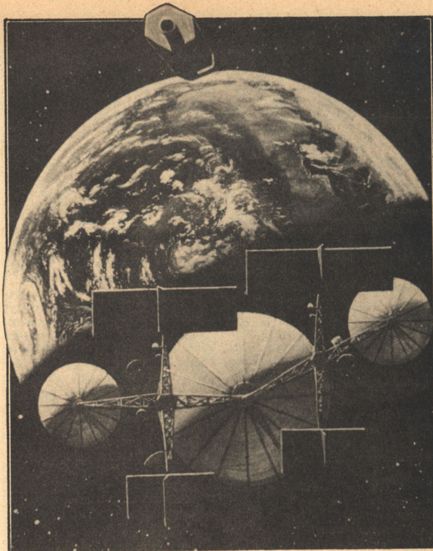
ORBITAL ANTENNA FARM—View from behind a large orbital antenna. Large square panels are solar power array, disks are direct broadcast antennas. Station would have links to other platforms in geosynchronous orbits, providing worldwide coverage. Deployment of these huge stations would be facilitated by the use of low-cost nuclear-powered spaceships. Artwork by David Egge; copyright Foundation, 1977.
