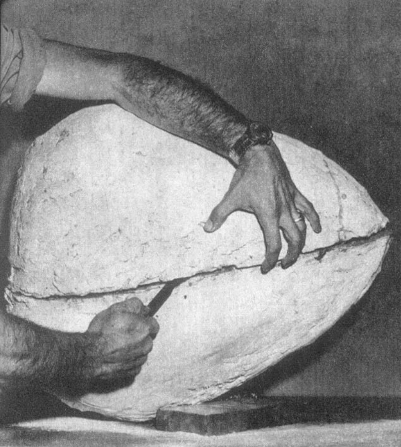
Step 3: Ticklish operation. Plaster mold is carefully pried apart.
