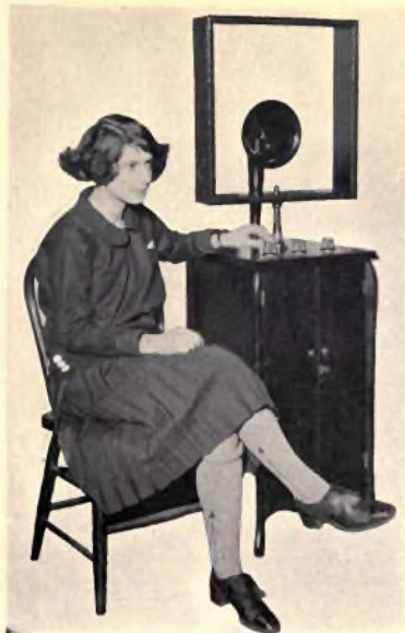
The author's "Radiotrol." This machine was built late in 1921, and is the first radio machine of its class to take on the appearance of a piece of furniture. The Radiotrol, now used in the author's home employs neither antenna nor ground, the reception being made by the loop shown in the engraving. The music, as well as entertainment, from WJZ, Newark, N. J., although twelve miles distant, comes in so loud that the sounds can be heard all over the apartment.
