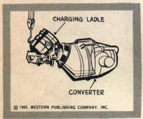
Melted iron is poured from a charging ladle into the pear-shaped converter. It is then turned upright and the air is forced in.
