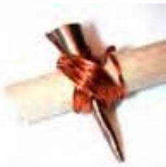
a handmade kistka using a piece of copper shaped into a cone and wired onto a dowel rod.
